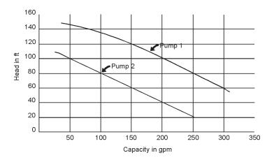
6. C) 200 gpm at 140 ft. head is the "best" answer For SERIES pumps, add HEAD, not GPM. In this case we find that at 200 GPM, Pump 1 is producing 100 FT of HEAD and Pump 2 is producing 40 FT of HEAD. This is the only one of the choices that works for these pumps.
