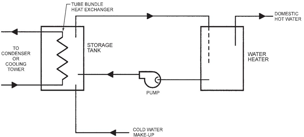
**Figure 7-4 Condenser Water Heat Recovery with Storage Tank**
