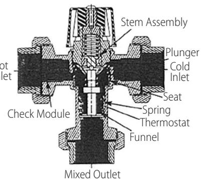
Figure 6-17 Temperature Mixing Valve
