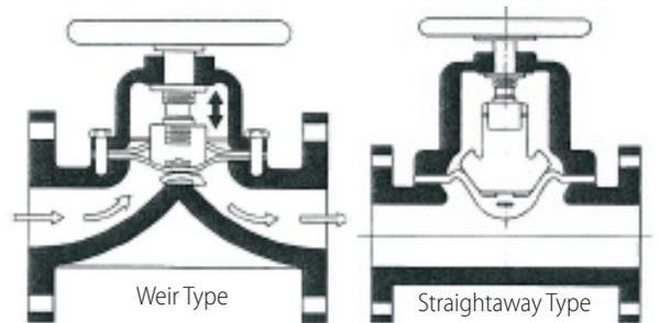
**Figure 6-10 Diaphragm Valves**
