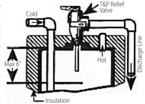
Figure 6-16 T&P Relief Valve Installation on a Water Heater
