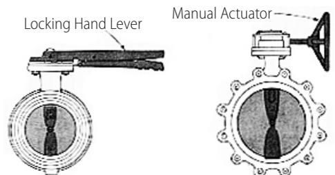
**Figure 6-8 Butterfly Valve Actuators**
