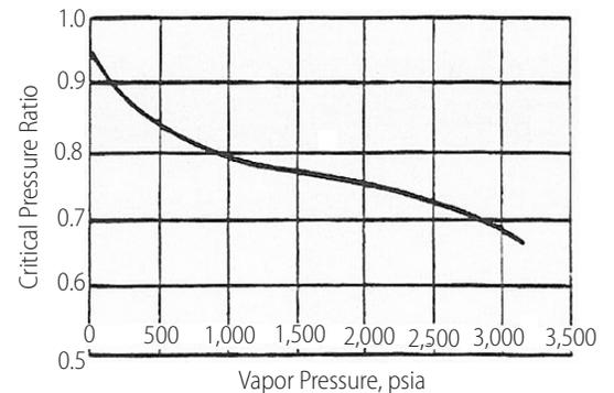
**Figure 6-19 Critical Pressure Ratio**
