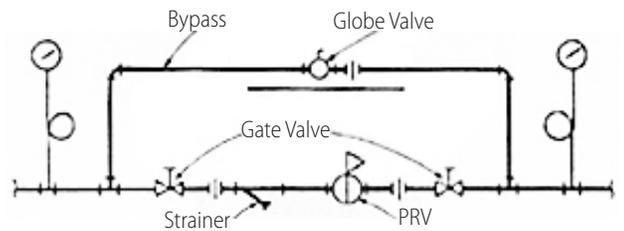
Figure 6-15 Typical PRV Assembly
