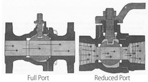
**Figure 6-7 Full-Port and Reduced-Port Ball Valves**
