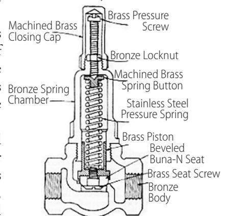
**Figure 6-13 Pressure-Regulating Valves**
