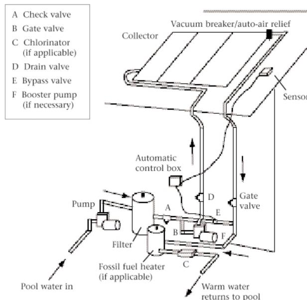
**Figure 10-4 Solar Pool Heating System**
