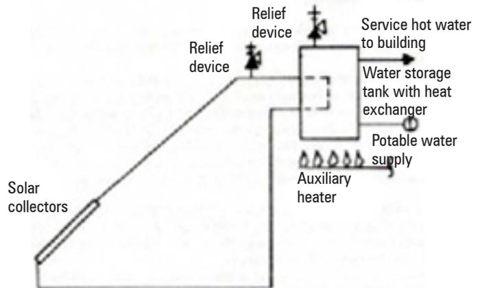
**Figure 10-6 Indirect Thermosiphon-Type Solar-Assisted Service Water Heating System**
