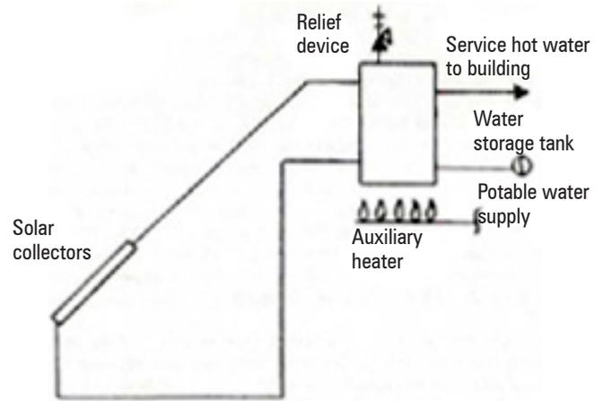
**Figure 10-5 Direct Thermosiphon-Type Solar-Assisted Service Water Heating System**
