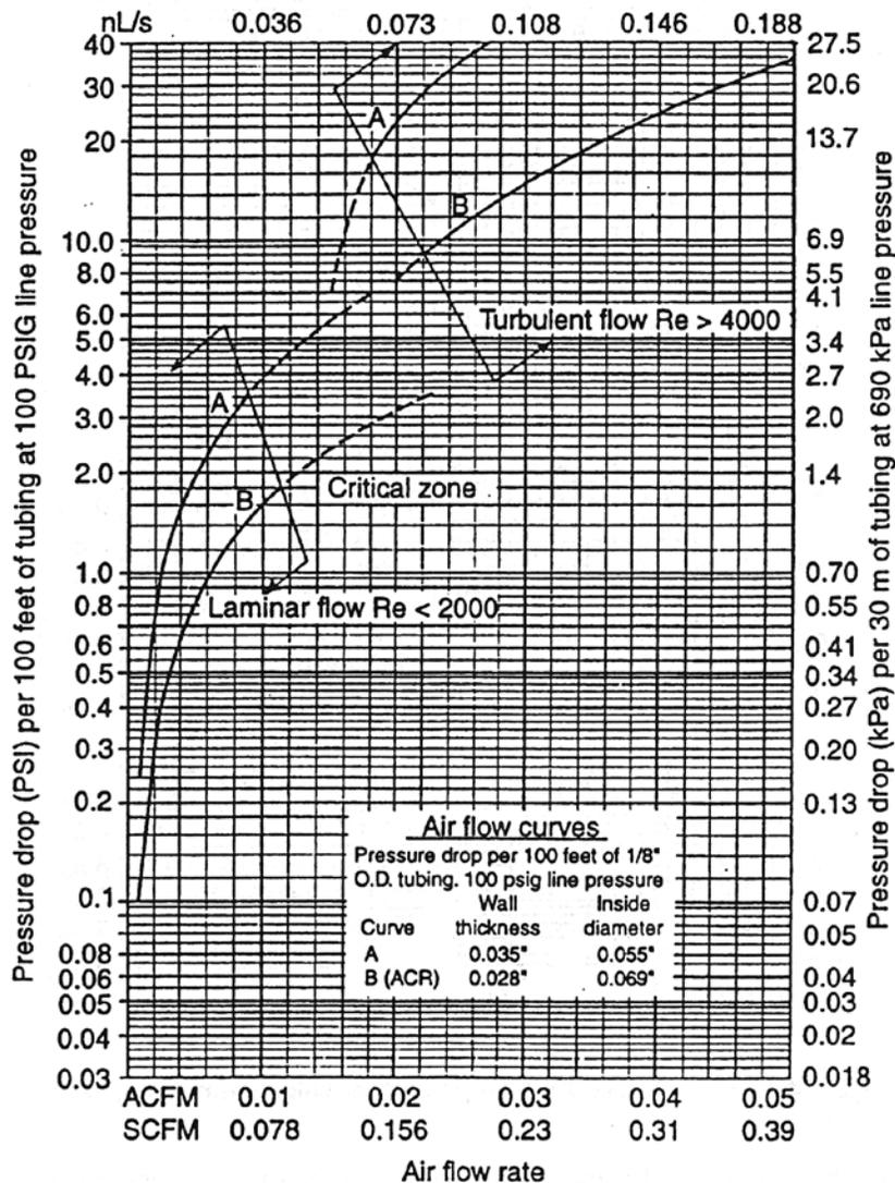
Figure 12-8 Sizing 1/8-inch OD Capillary Piping and Tubing
