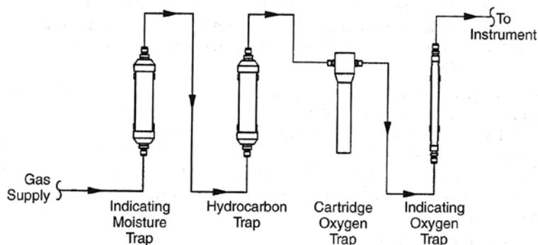
Figure 12-5 Typical Purifier Arrangement
