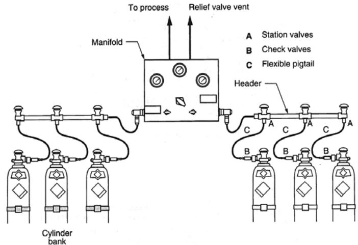
**Figure 12-3 Typical Manifold Assembly**
