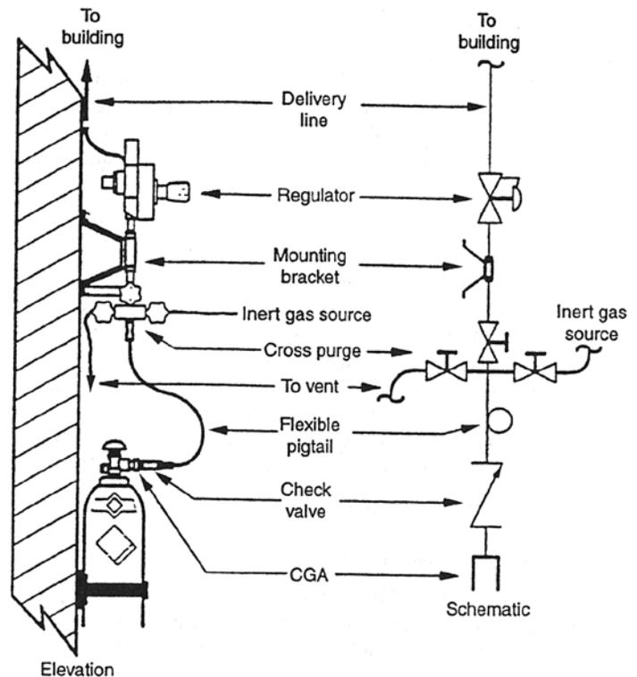
**Figure 12-7 Regulator Purging Arrangement**
