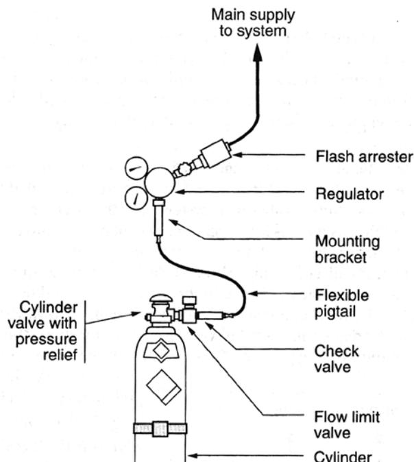
Figure 12-2 Cylinder Components
