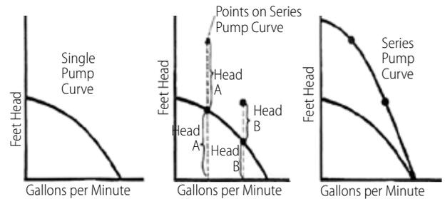
Figure 4-21 Series Pump Curve Construction
