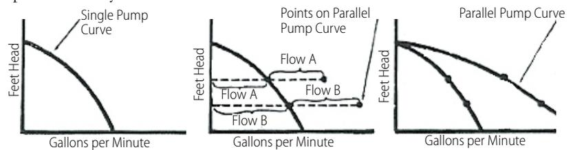
Figure 4-22 Parallel Pump Curve Construction
