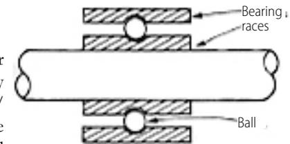
Figure 4-4 Ball Bearing
