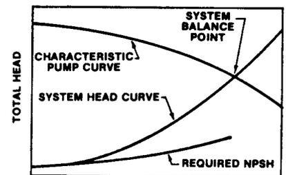
**Figure 4-18 Typical Pump Curve Crossing a System Head Curve**
