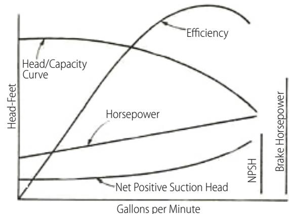
**Figure 4-14 Pump Efficiency**
