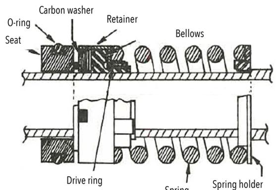
Figure 4-3 Mechanical Seal
