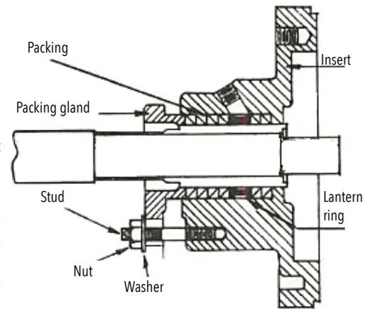
Figure 4-2 Packing Seal
