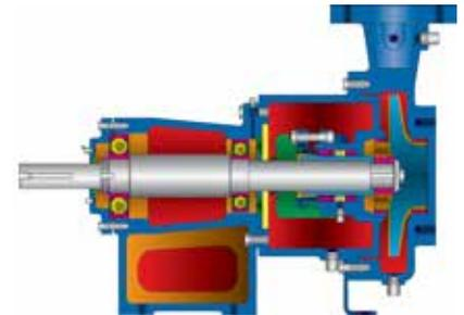
**Figure 4-6 Single-Suction Volute Pump with End-Suction Design**
