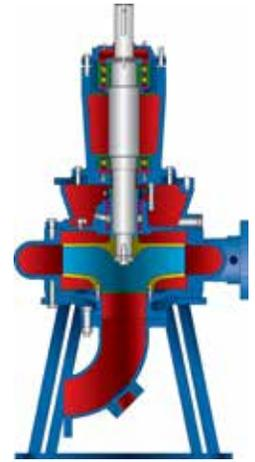
**Figure 4-10 Dry Pit Mounted Vertical Pump**
