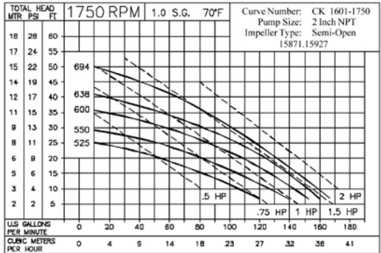
Figure 4-19 Typical Pump Curves and Power Requirements
