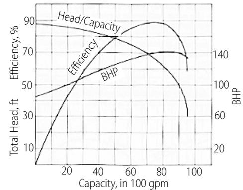
**Figure 4-16 Non-Overloading Power/Capacity Curve**
