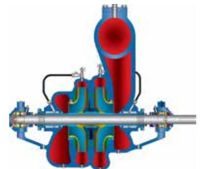
**Figure 4-9 Horizontal Split-Case Pump**
