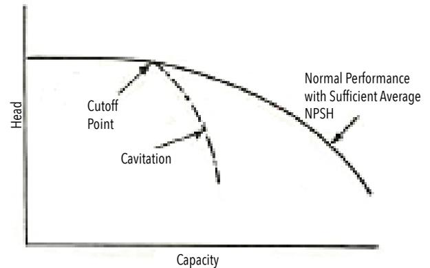
Figure 4-20 Cavitation’s Effect on Pump Capacity
