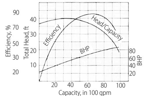
**Figure 4-17 Overloading Power/Capacity Curve**
