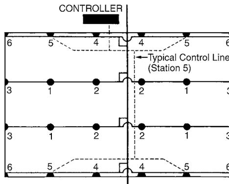
1. Main can supply four 20 gpm (75.7 L/min) sprinklers at one time.
