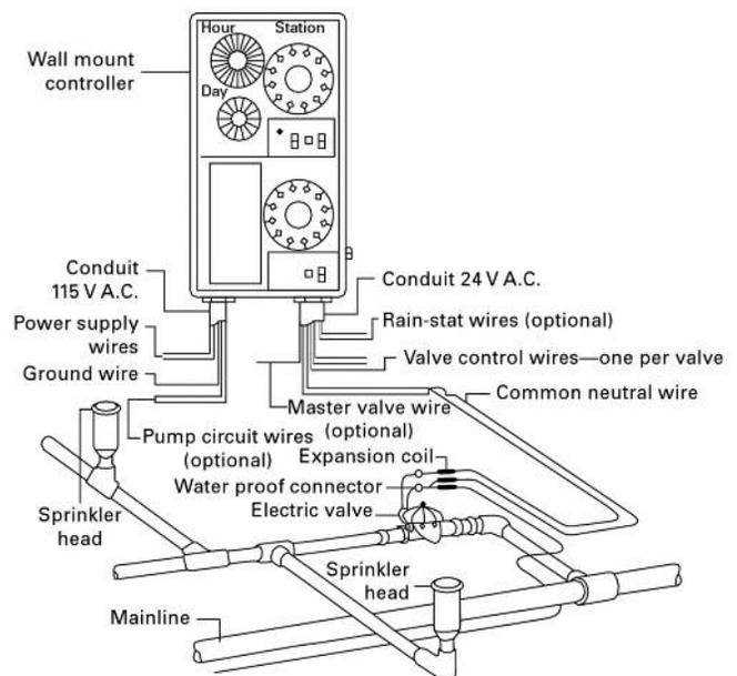
**Figure 4-9 Surface-Mounted Irrigation Sprinkler Controller**
