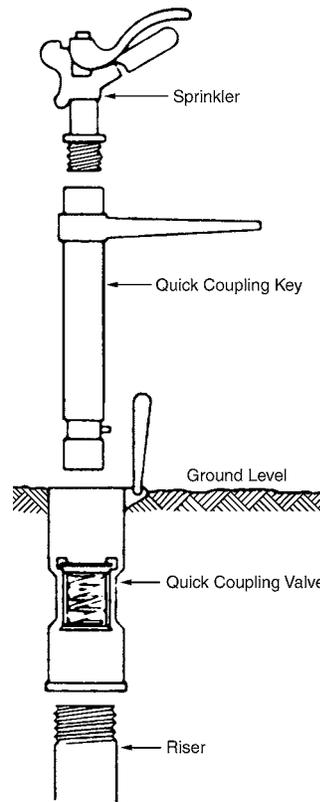
**Figure 4-2 Quick-Coupling Valve**
