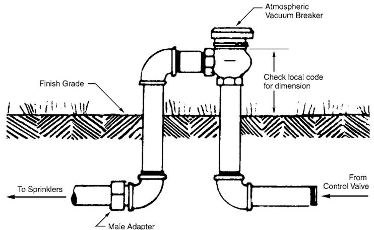
**Figure 4-8 Installation of an Atmospheric Vacuum Breaker**
