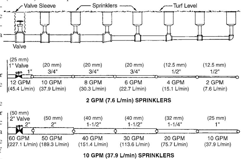
**Figure 4-1 Examples of a Block System**
