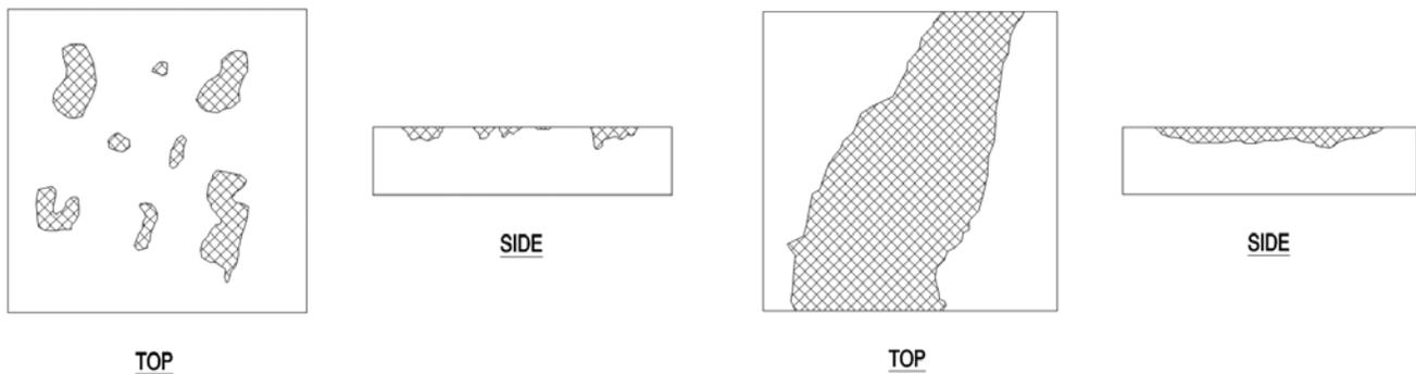
**Figure 8-9 (A) Plug-Type Dezincification (B) Layer-Type Dezincification**
