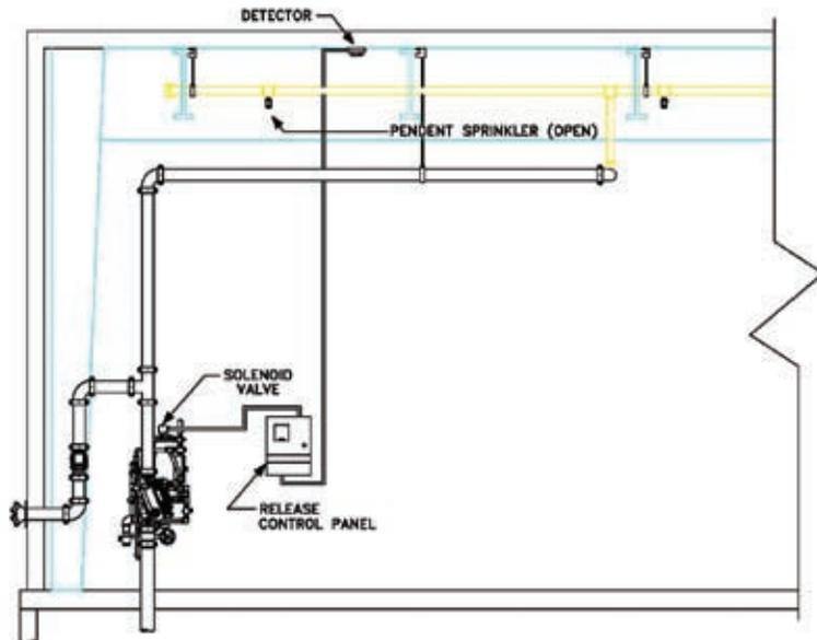
Figure 4 Diagram of a typical deluge service entrance
