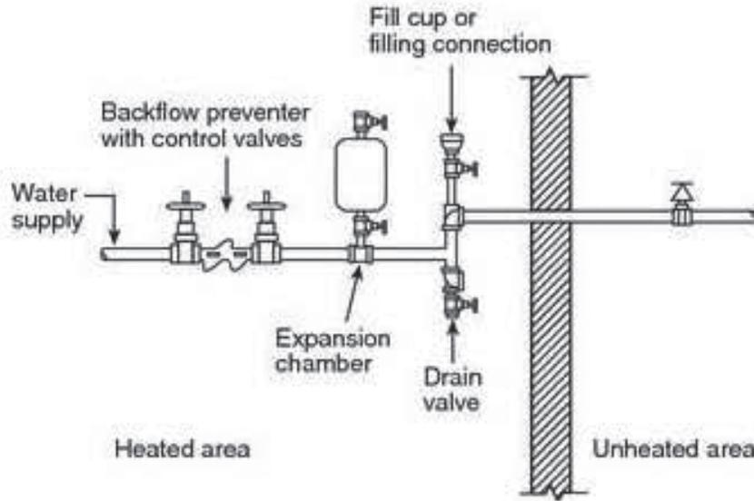
Figure 5 Diagram of a typical antifreeze system
