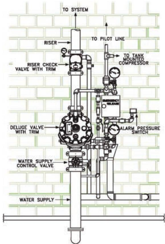
Figure 3 Diagram of a typical preaction service entrance
