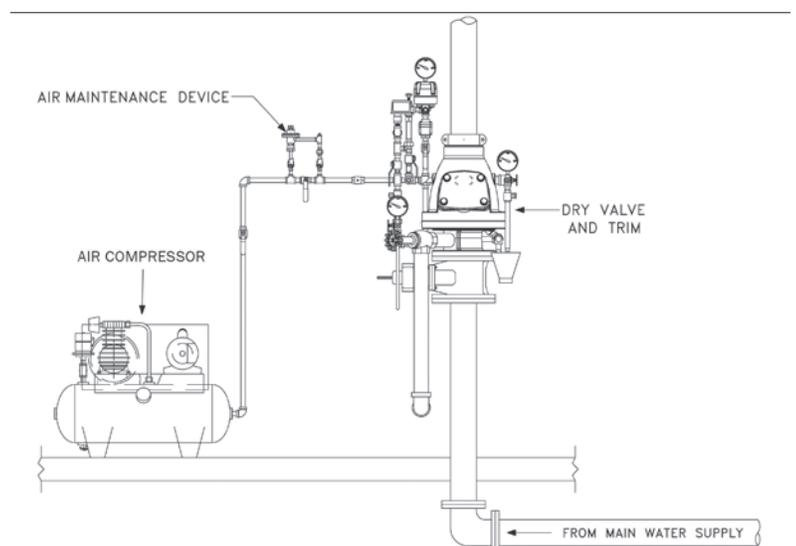
Figure 2 Diagram of a typical dry-pipe service entrance
