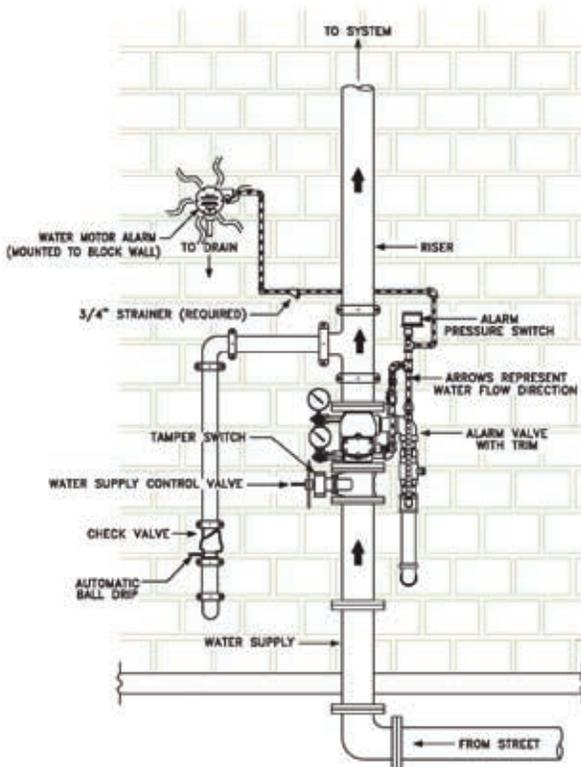
Figure 1 Diagram of a typical wet-pipe service entrance
